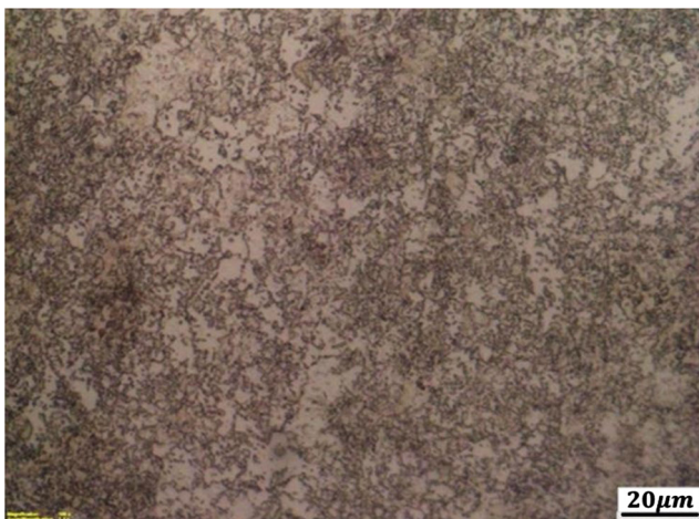
Fig. 1 Micrograph of the investigated steel grade 980
